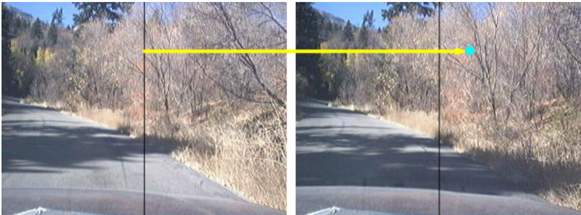
Figure 28 - Hand Annotation of two images 10 frames apart Black lines are the middle of the image; The area in the middle of the left frame (10 frames previous) is marked with an Aqua dot in the right frame (current frame); The yellow arrow indicates the movement of corresponding area from frame to frame
