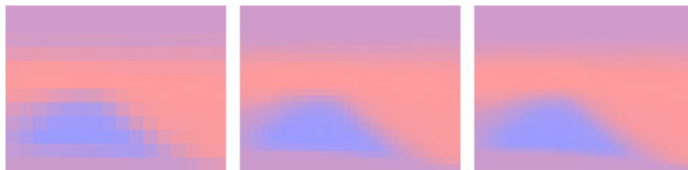
Figure 41 - Probability Grid Granularity Red – Probable Obstacle; Blue – Probable Safe; Purple – Unsure Left: 20x20 pixel cells; Center: 5x5 pixel cells; 1x1 pixel cells
