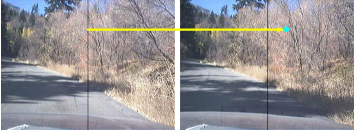
Figure 11 - Hand Annotation of two images 10 frames apart Black lines are the middle of the image; The area in the middle of the left frame (10 frames previous) is marked with an Aqua dot in the right frame (current frame); The yellow arrow indicates the movement of corresponding area from frame to frame
