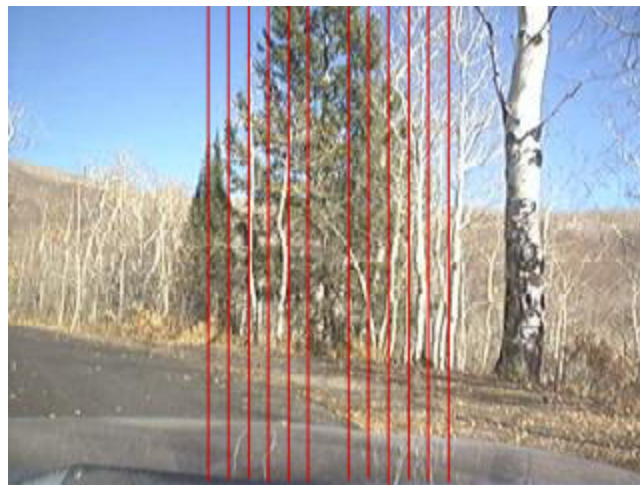
Figure 10 - Discrete Ranges of Pixels These provide a discrete measurement and help reduce the effect of noise
